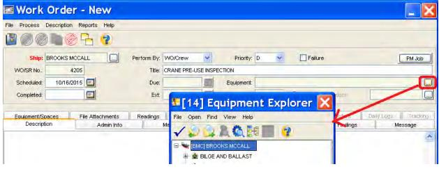
In the Equipment Explorer, click the plus sign to the left of "Deck Equipment". That will open the deck equipment list. Click the box next to Crane-back deck to select. Then click to blue check mark at the top of the window to confirm.
